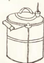
ments are simply that the interior vessel shall be raised about half an inch above the bottom of the other, and that the water shall reach nearly or quite as high as the milk. The apparatus is then heated on a range or stove until the water reaches a temperature of 155° Fahrenheit, when it is removed from the heat and kept tightly covered for half
