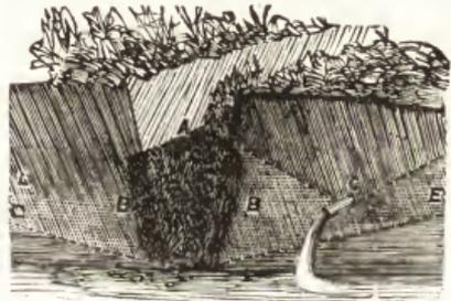
*Open Ditch Drain Contrasted with Tile Drain.*
