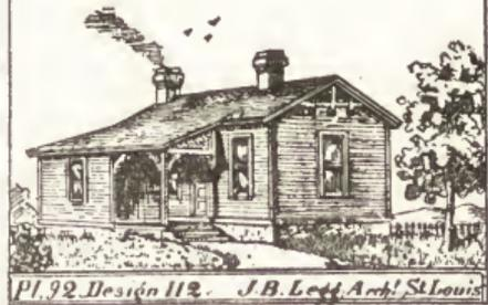
columns are square and without base or cap, running up to the eaves of roof with a spandrel in front intended to be shingled. Molded brackets are placed on the posts in the angles. The porch is large and will shade the sunny side of the house. The approximate cost of the building would be about \$1,200.
